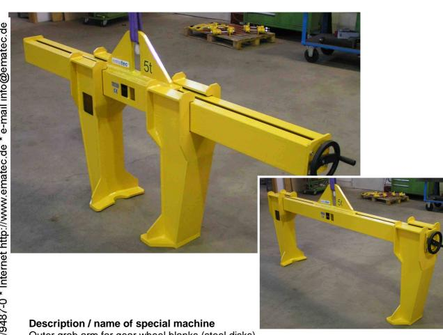
Outer grab arm for gear wheel blanks (steel disks)
