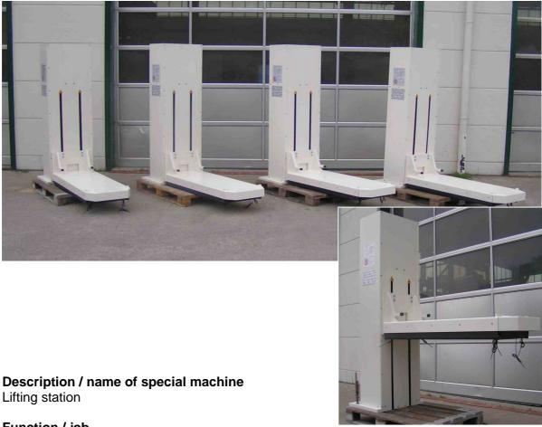
Function / job Ergonomical provision of work piece boxes. For the feeding of a manufacturing line
