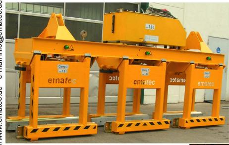
**Description / name of special machine** 3-fold slab tongs, hydraulically powered
