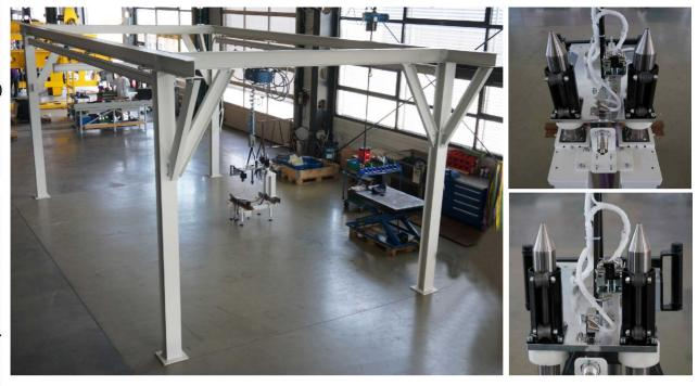
**Description / name of special machine** Gantry with rope balancer and pneumatic gripper
